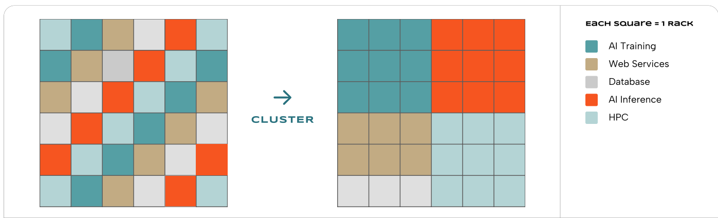
Figure 1: Workload clustering transforms a chaotic mix of job types (left) into organized zones where similar workloads are co-located (right). This enables zone-specific cooling and reduces resource contention.
